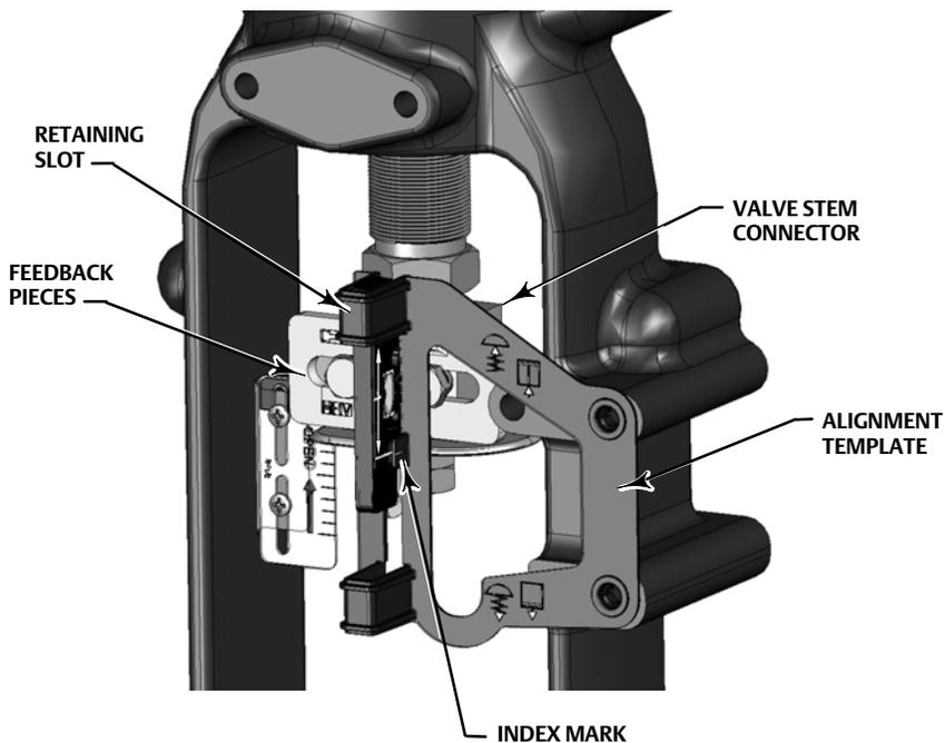
1. Tighten the fasteners and remove the alignment template.
