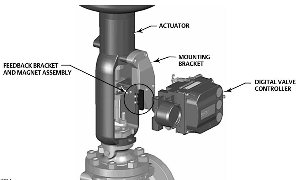
2. Attach the mounting bracket to the actuator.
