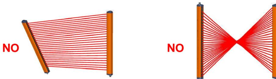
Fig. 14 – Light curtain alignment
